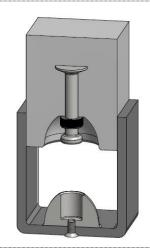
The steel recess formers SBK and SBKM are always used in combination with a rubber ring. The rubber ring ensures that the anchor fits snugly in the former. Moreover, the rubber ring prevents concrete pouring into the recess former.
